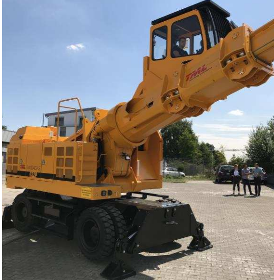
UNIDACHS 640P with tiltable driver's cabin
