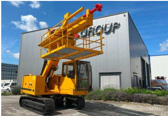
UNIDACHS 423 - BOF Tap hole drilling and sleeve setting machine
